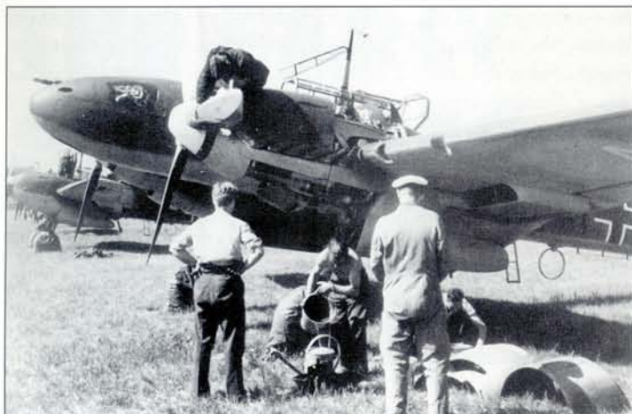
The first Gruppe to be equipped with the Bf 110C was I.(Z)/LG 1, the operational trials unit based at Barth on the Baltic coast. As with any new aircraft entering service for the first time, the Bf 110 was beset by a number of small technical problems, as this photograph clearly shows – the cowlings have been removed to allow the groundcrew better access to the troublesome port DB 601 engine of aircraft L1+A12 of 2. Staffel
